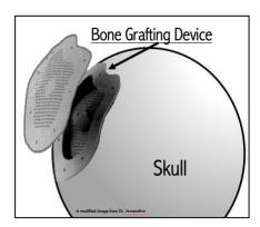
Figure 1: Illustration giving an example of the bone grafting device implanted in a skull. Note that it is porous to allow vasculature access, it has an overhang for screws to attach the device to the skull, and a reservoir for storing osteogenic materials.
