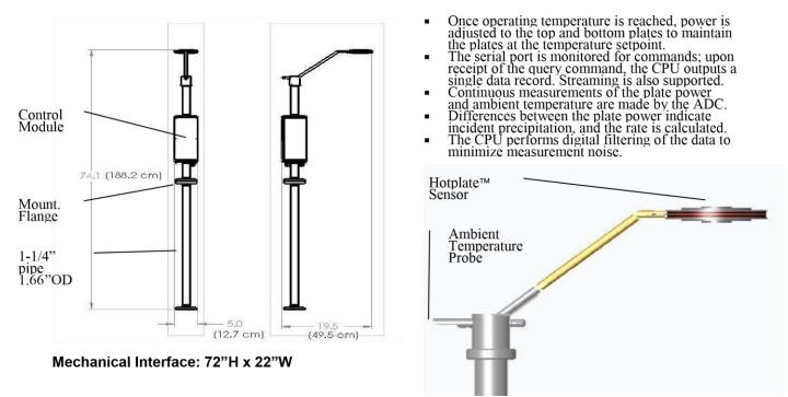
FIG. 2: Schematic of TPS-3100 and basic principles of device functionality (Yankee Environmental Systems, 2005)
