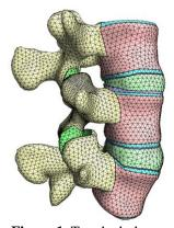
Figure 1. Tetrahedral Meshed Lumbar Vertebrae: The base laminectomy model used in this study.
